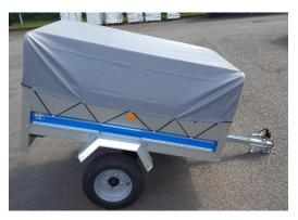
Ensure the cover is fully secured to the trailer by hooking the elastic cord under the clips found on the body of the trailer.
